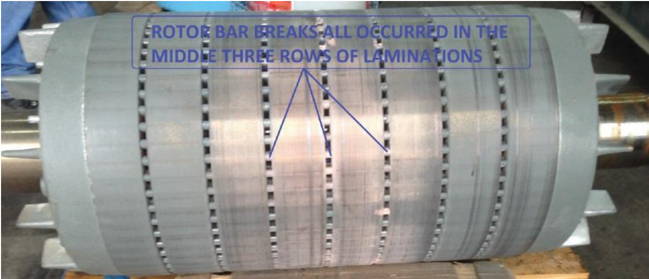
Rotor bar breaks all occurred in the middle three rows of laminations.
